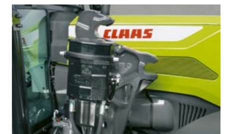
FITLOCK system for rapid attachment/removal and MACH quick-release coupler for electric and hydraulic connections
