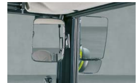
As well as the large standard mirror, a wide-angle mirror is also available for enhanced road safety
