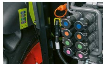
The rear connections are easy to identify thanks to colour-coding and adjacent stickers
