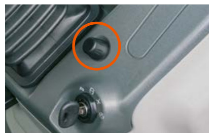
Use the rotary switch beside the steering column to navigate easily through the menu
