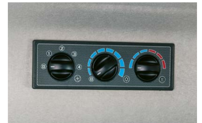
The controls for the air conditioning are within easy reach on the right-hand side of the cab roof liner
