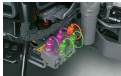
Up to four hydraulic connections and a free-flow return are available at the front
