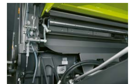
The large stone trap can be opened and emptied easily.
