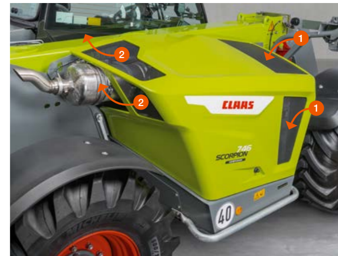
▲ Air is drawn in from the clean area at the front (1) and discharged upwards at the rear (2). This helps to keep animals calm and at the same time reduces dust.
