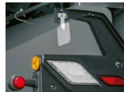
Sensor for automatic discharge direction adjustment
