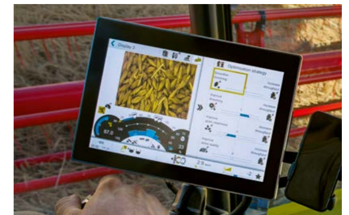
Intelligent control by CEMOS AUTOMATIC via CEBIS
