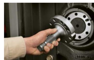
The PTO stub can be changed easily
