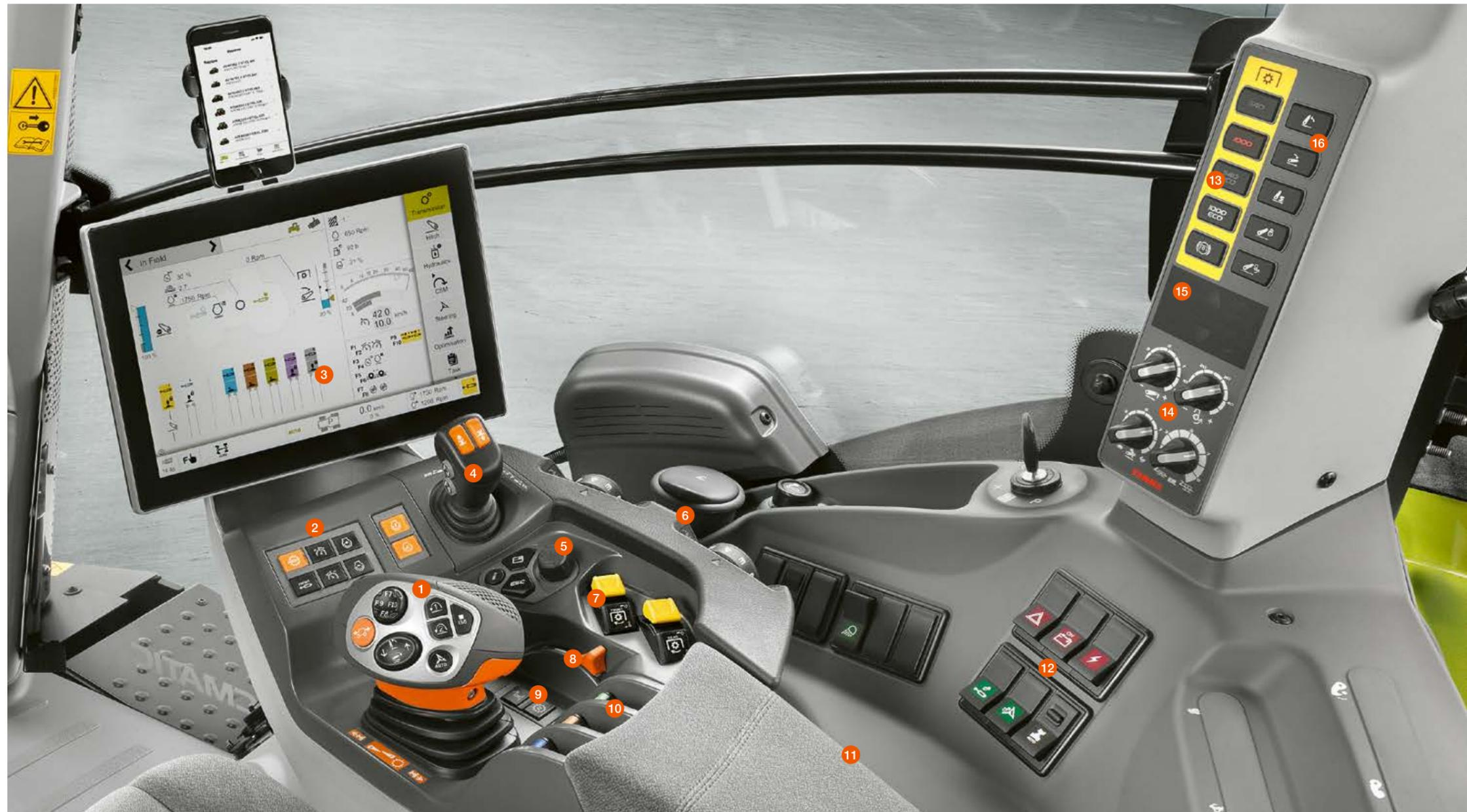
The height and position of the armrest can easily be adjusted to the driver's requirements.
