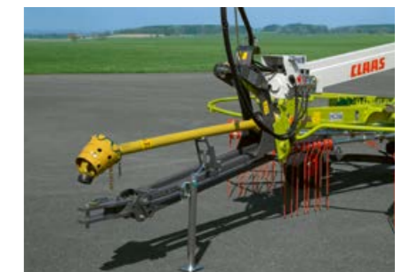
Parallelogram drawbar is optional on the LINER 700 TWIN and standard on the LINER 800 TWIN.
