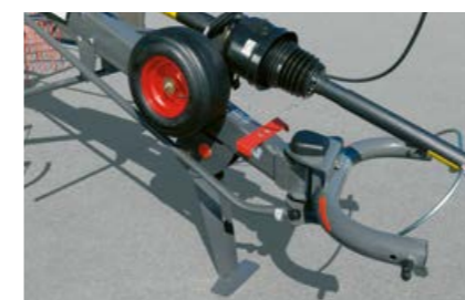
The flexible inverted U-frame hitch with lateral oscillation allows a steering lock angle of up to 80°.
