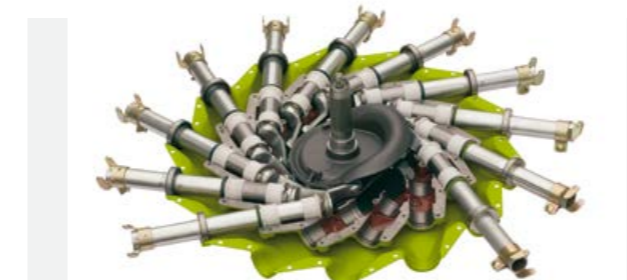
Maintenance-free reliability: the core component of the LINER is the cam track running in an oil bath.
