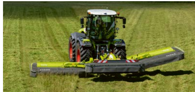
Individual mower unit lift at the headland
