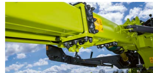
Two hydraulically controllable telescopic arms with continuous adjustment for optimal overlapping in the DISCO 1100 COMFORT
