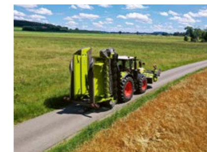
Compact transport position for safe road travel
