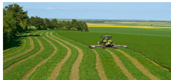
Optimum results even in curves, thanks to maximum overlap (up to 60 cm)
