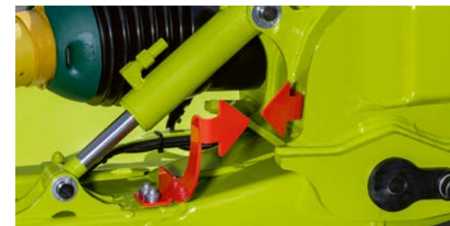
Easy adjustment of central frame height: just line up the arrows
