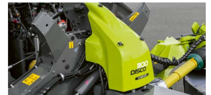
Compact, robust headstock with integrated ACTIVE FLOAT suspension system as standard
