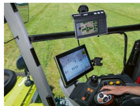
Comfortable operation, for example via a range of ISOBUS terminals and the ISOBUS function keys on the control lever
