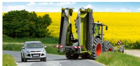
Less than 4.0 m: compact transport position with generous ground clearance in both BUSINESS models
