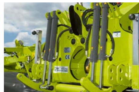
The standard lift and suspension rams of the ACTIVE FLOAT suspension system provide reliable sward protection
