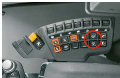
One switch for the entire folding process.
