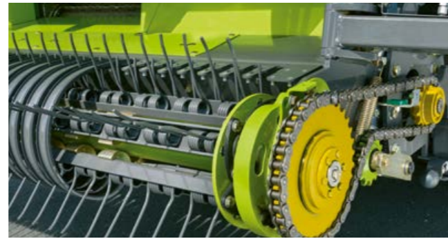
Robust pick-up reel for efficient crop intake.
