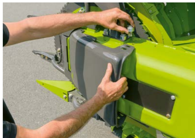
Skids with two height settings.
