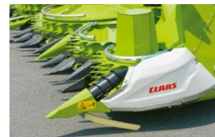
Hydraulically driven laid maize point.
