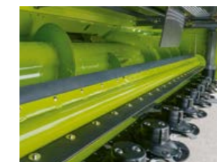
DIRECT DISC 600 P / 500 P with height-adjustable paddle roller, optionally with hydraulic operation.
