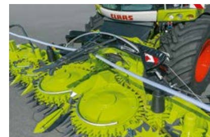
Compact deployment with an unrestricted view of the ORBIS during harvesting. Transport protection remains stowed securely on the machine.
