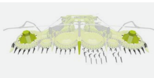
Laid maize cones, guide elements and tip extensions available as additional equipment.
