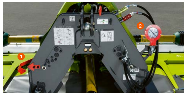
1 Working height setting 2 ACTIVE FLOAT pressure gauge
