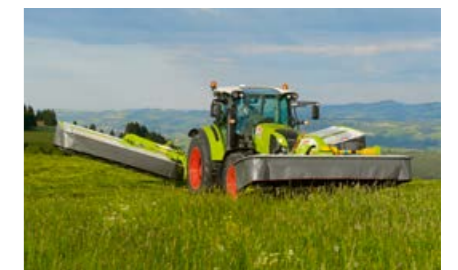
Compact headstock at the front linkage gives the mower generous ground clearance at headlands
