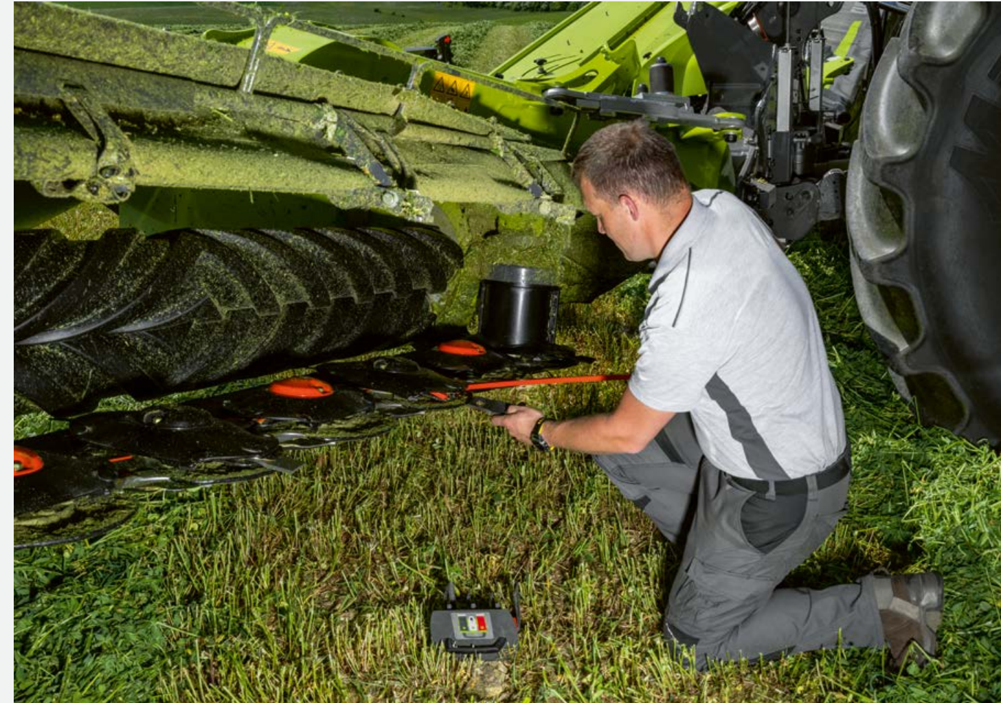
Spare knives are stored in a weatherproof box on the mower, along with an integrated fitting lever – making knife changes in the field quick and straightforward.
