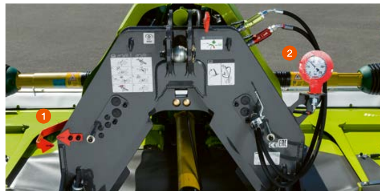
1 Working height setting 2 ACTIVE FLOAT pressure gauge
