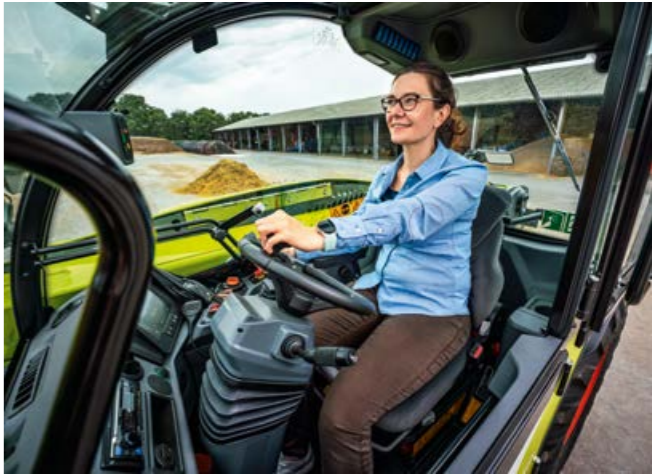
▲ Informative terminal. Key parameters and the current operating status of the machine and units are always in view. The sub-menus are easy to understand. A 7" colour display is also available as an option.
