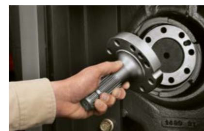
The PTO stub can be changed easily
