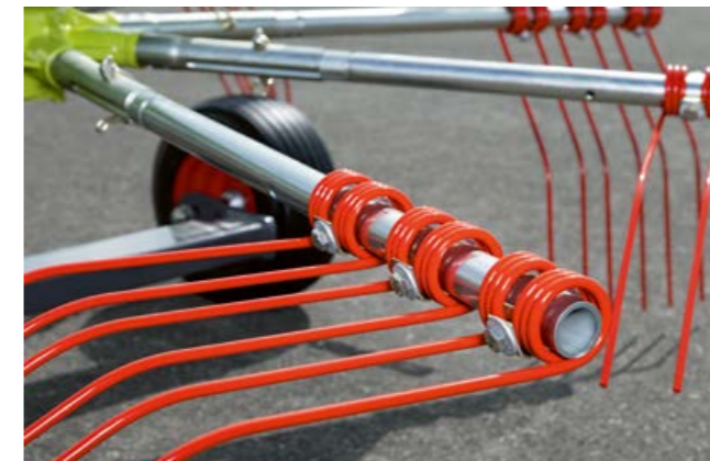
Tool-free tine arm removal.
