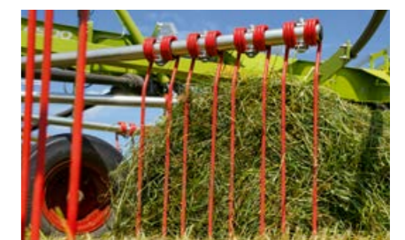
Silage tines for gentle forage handling.
