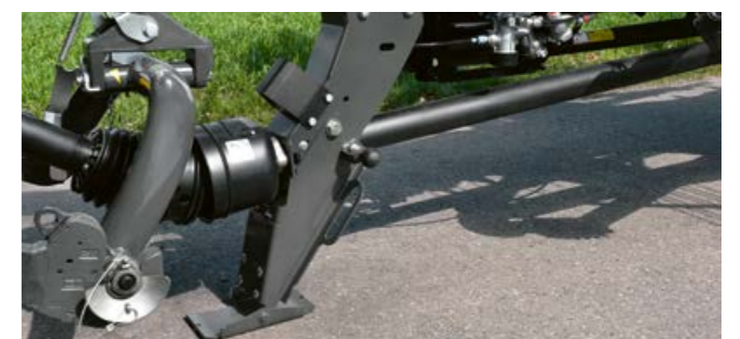
Semi-automatic parking stand. All LINER four-rotor swathers have a cleverly designed semi-automatic stand which can easily be operated with just one hand.
