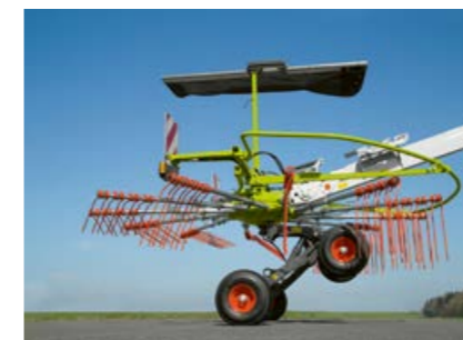
Generous lift height for driving over swaths at the headland: up to 50 cm in the LINER 700 TWIN.
