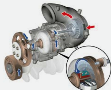
Turbo-compound technology for OM 473 LA
