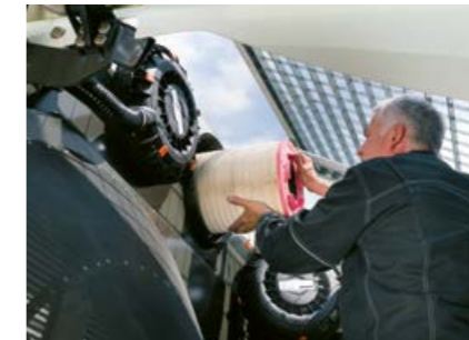
Air filter change without tools
