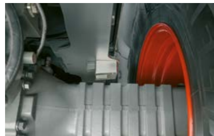
To allow even very large tyres to be used in agricultural applications, the oscillation travel of the rear axle can be limited.
