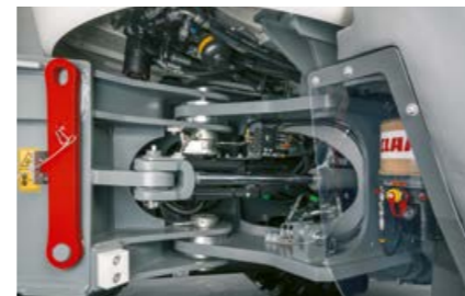
The articulated joint with a 40° angle of articulation makes the TORION agile and easy to manoeuvre.
