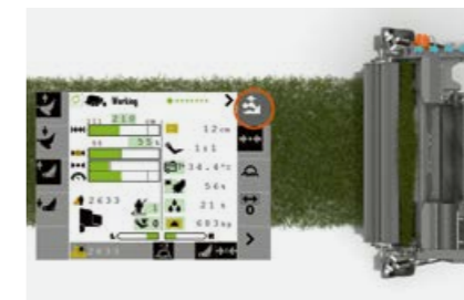
The hydraulic PFS intake is easy to adjust from the tractor seat.
