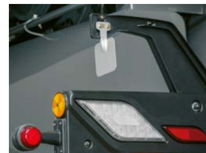
Sensor for automatic discharge direction adjustment
