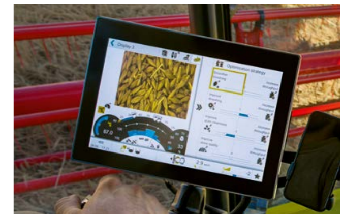
Intelligent control by CEMOS AUTOMATIC via CEBIS.
