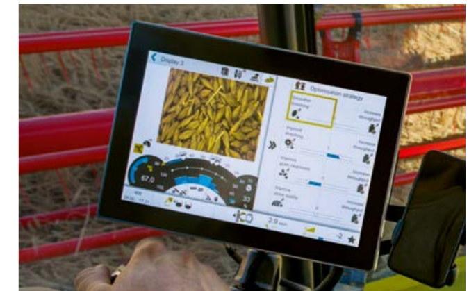
Intelligent control by CEMOS AUTOMATIC via CEBIS.
