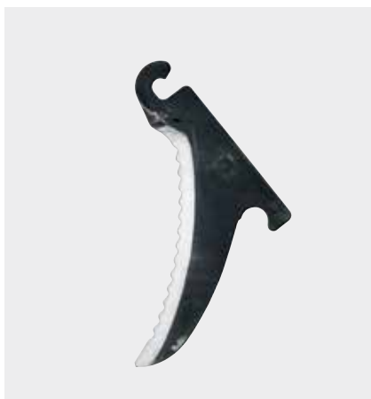
Properly sharpened knife: ideal, sharply defined scallop pattern.
