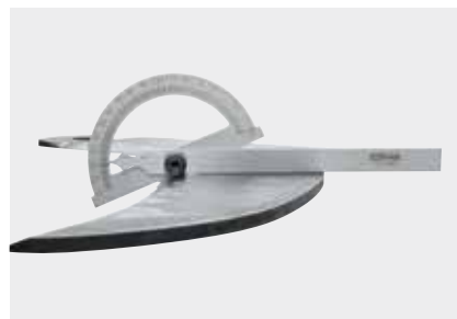
Incorrectly sharpened knife: angle approx. 22°.
