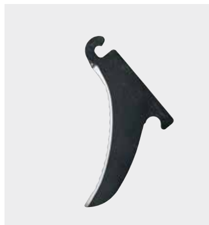
Incorrectly sharpened knife: less defined scallop pattern.
