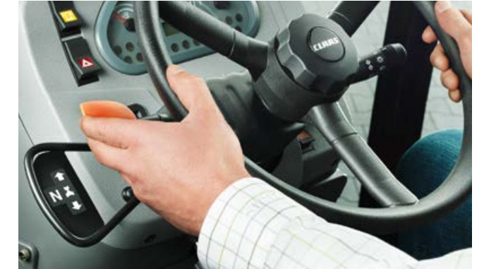
1 REVERSHIFT lever for rapid and comfortable turning manoeuvres, particularly at headlands or when stacking boxes.
