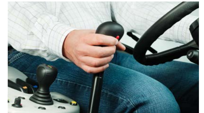
1 REVERSHIFT lever for rapid and comfortable turning manoeuvres, particularly at headlands or when stacking boxes.
