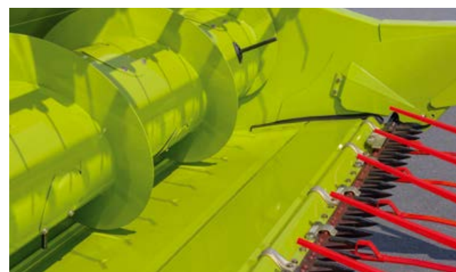
Cutterbar table extended – grain (+100 mm)
