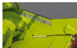
The operator in the cab has a perfect view of the position indicator for the cutterbar tray
