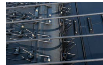
The tines ensure the crop is picked up and passed on quickly
