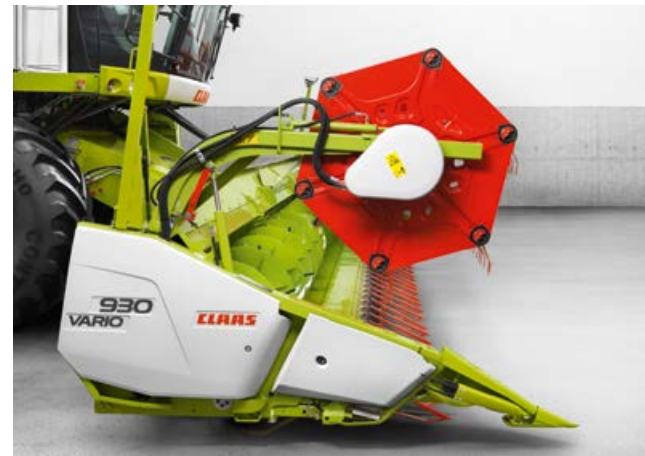
Cutterbar table retracted – grain (-100 mm)
