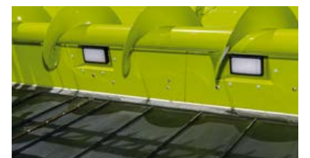
Powerful work lights illuminate the cutterbar and trough perfectly
