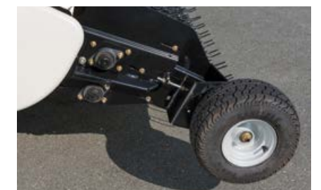
Castor guide wheels limit the depth
