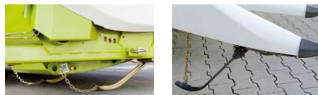
Sensor bands detect the position of the front attachment for AUTO CONTOUR and CONTOUR
