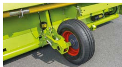
Stabiliser wheels guide the cutterbar smoothly under all conditions
