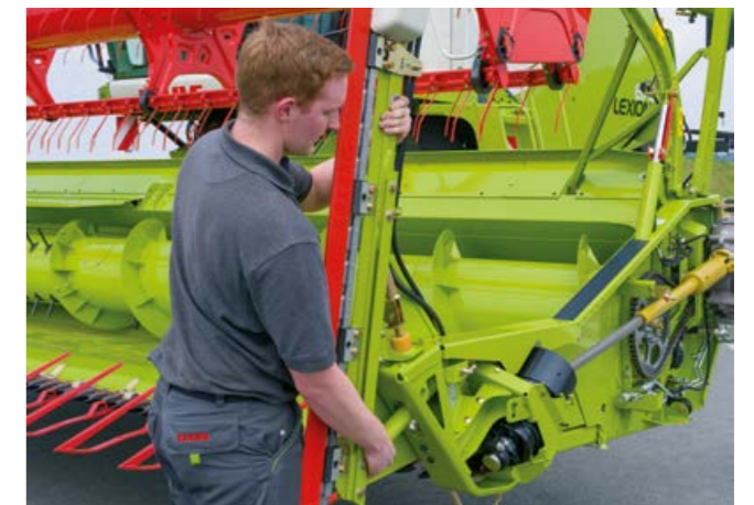
Rapeseed knives fitted by means of quick-release mounting system
