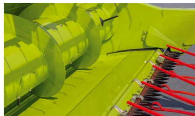
Cutterbar table extended – grain (+100 mm)
