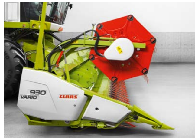
Cutterbar table retracted – grain (-100 mm)
