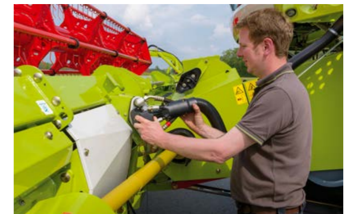
Multicoupler and central locking make for extremely convenient operation
