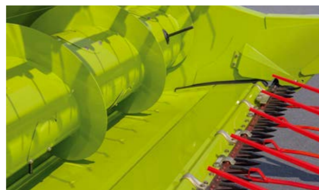
Cutterbar table extended – grain (+100 mm)
