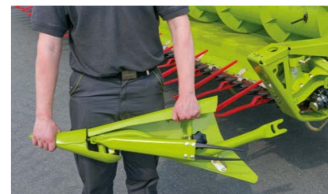
Quick and easy replacement of dividers
