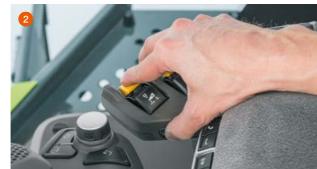
Reversing via CMOTION (1) or by simultaneously pressing the toggle switch and the reversing button (2)
