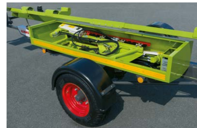
Locking transport container for rapeseed equipment
