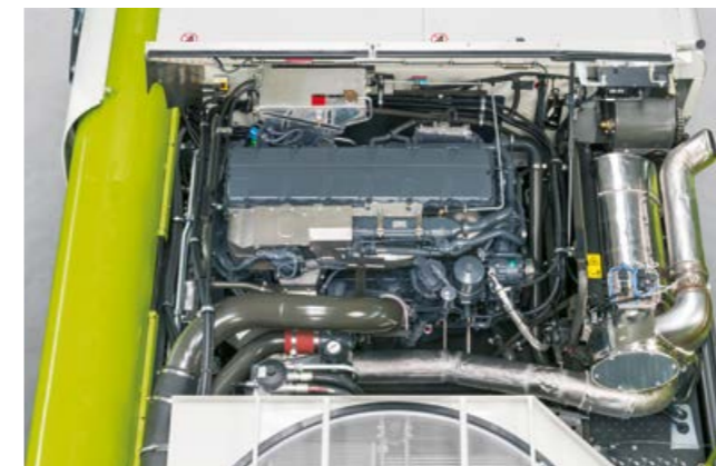
MAN D42 with 581 kW / 790 hp for LEXION 8900
