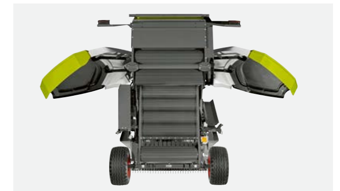
The fixed-chamber design concept of the ROLLANT 620.
