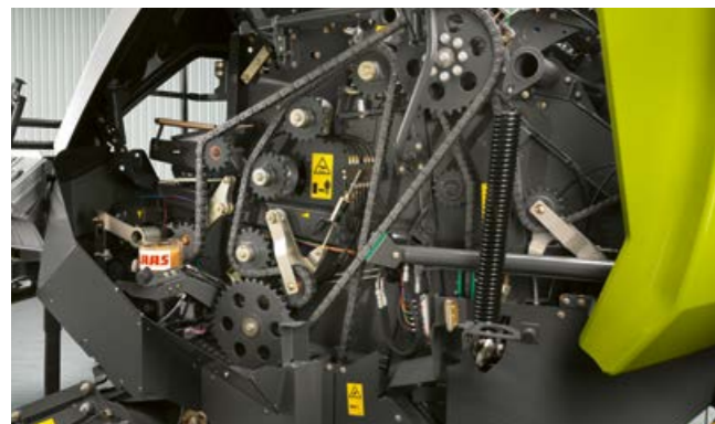
Power-efficient drive concept.
