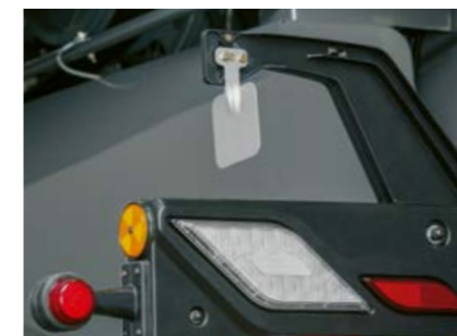
Sensor for automatic discharge direction adjustment
