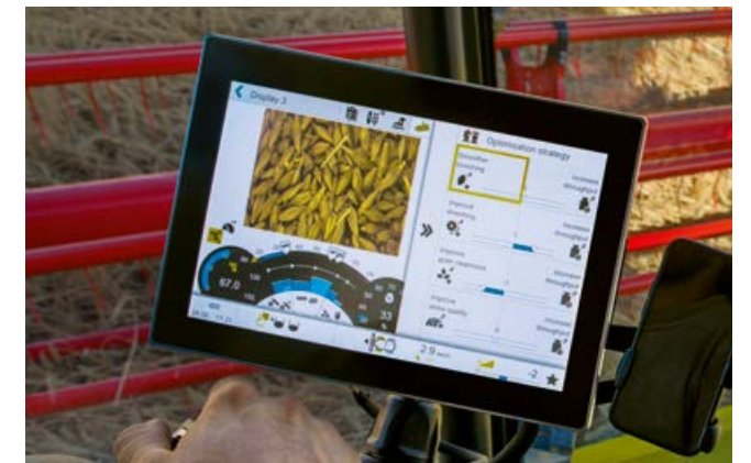
Intelligent control by CEMOS AUTOMATIC via CEBIS
