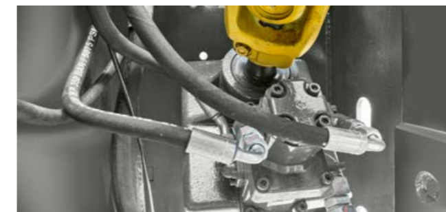
Two oil pumps supply hydraulic oil to the input transmission and the TURBO FAN knotter cleaning system.
