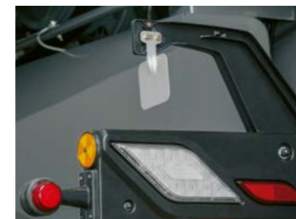
Sensor for automatic discharge direction adjustment.
