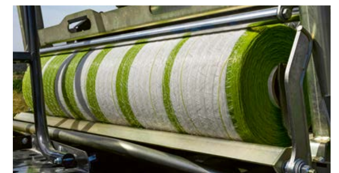
The new net wrapping system in the VARIANT 500 series is positioned 25 cm lower to allow easy cleaning of the net roll under the net brake.
