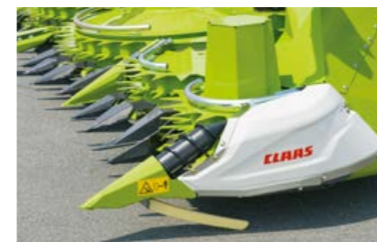
Hydraulically driven laid maize point.
