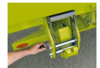
With the front attachment locked in place, it is possible to travel safely at up to 40 km/h.
