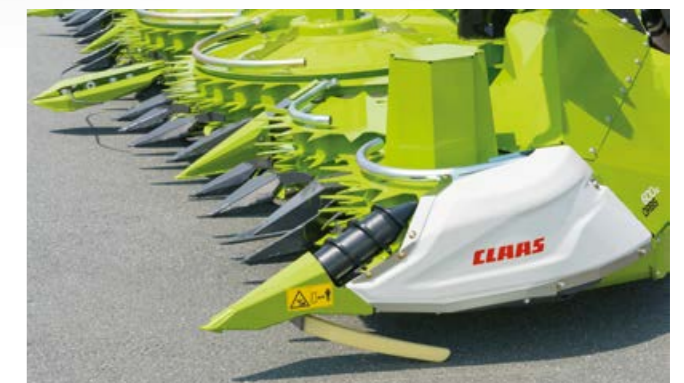
If required, the laid maize augers are driven hydraulically.
