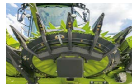
Robust guide fingers and dischargers under the cutting disc for problem-free operation.
