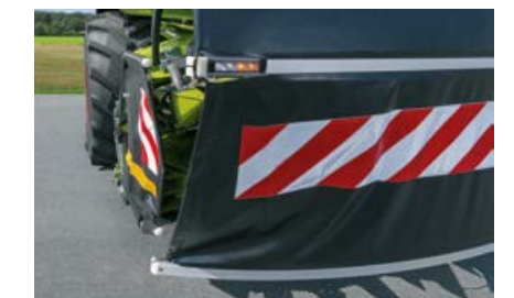
Side and front protection clearly visible with warning stickers. The LED lighting is fully integrated.
