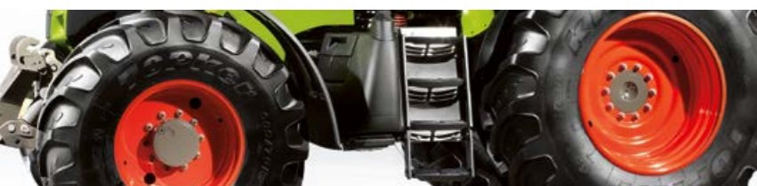
Well-positioned steps and handles provide safe and convenient access to the cab
