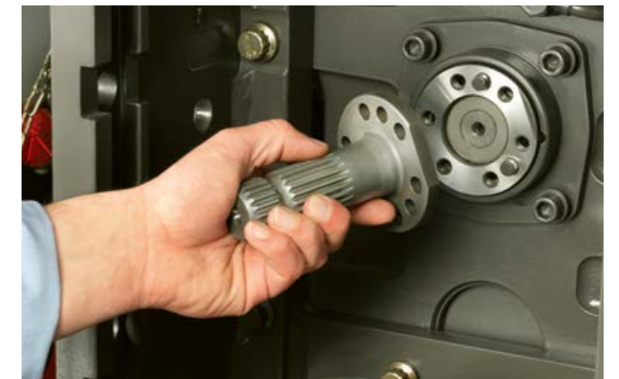
The PTO stub is easy to change.
