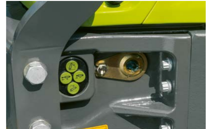
With electronic spool valves, the front linkage and additional spool valve can be controlled externally.
