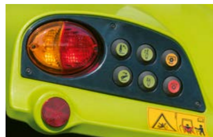
Controls for the rear linkage, electronic spool valve and PTO are available for both mudguards. The left mudguard has a holder for four lower link balls.
