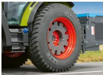
You can add up to 270 kg of ballast to the left rear wheel to offset the weight of the telescopic boom for safe, stable road travel
