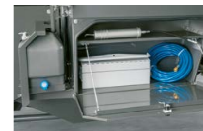
20 litres of water and a soap dispenser are available for hand washing when work is over.
