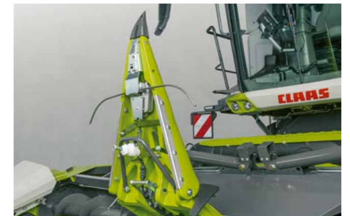
Two sensor bands each scan a row of maize.
