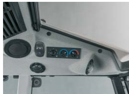
The heating and ventilation system has a four-stage fan and several adjustable air jets. A controllable air-conditioning system is also available.
