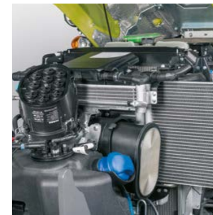
The PowerCore® air filter is located in easy reach under the bonnet at the front and reduces the cleaning interval
