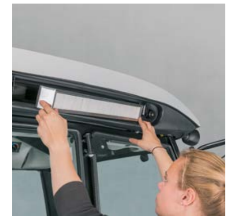
The cab air filter is easy to access from outside for cleaning and keeps the air in the cab fresh at all times
