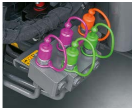
Up to four hydraulic connections and a free-flow return are available at the front to the right of the cab
