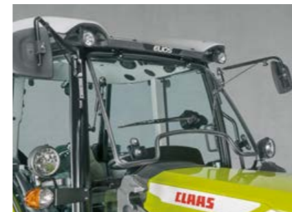
The front windscreen opens for natural ventilation
