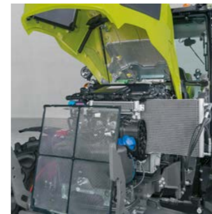
You can slide out the radiator and remove the radiator screen in no time for inspection and cleaning
