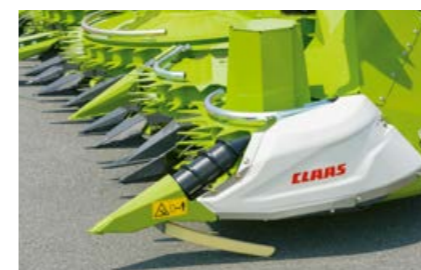
Hydraulically driven laid maize point.
