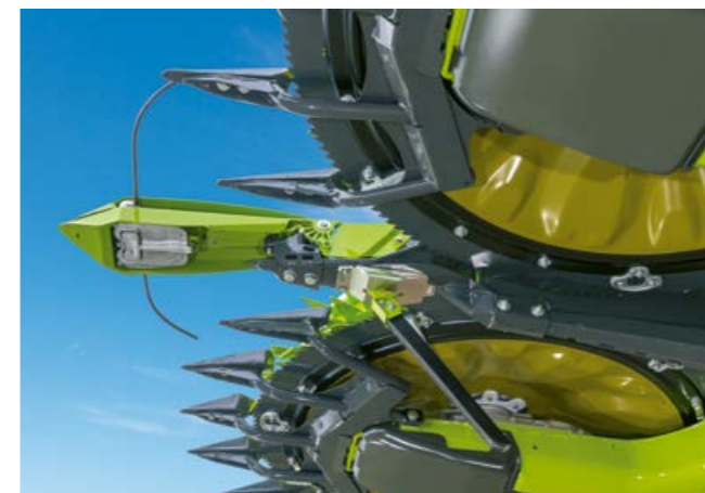
AUTO CONTOUR centre sensor, available for ORBIS 900.
