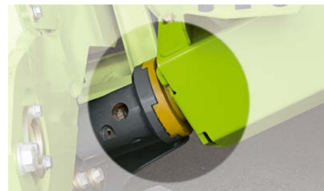
Power transmission via quick-release coupler.
