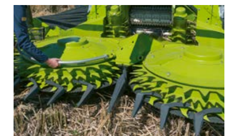
Removal of cob retainers increases crop flow performance.
