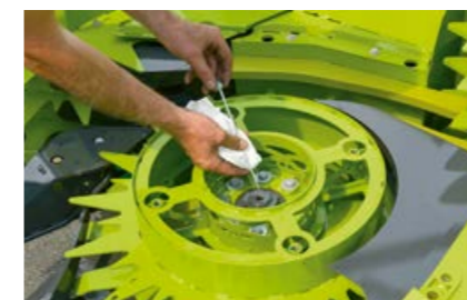
Dipstick to check oil level.
