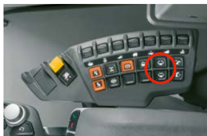
One switch for the entire folding process.
