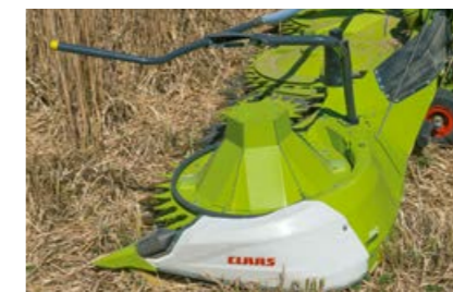
The large laid maize cone optimises the crop flow and prevents crop material from remaining on the transport disc.
