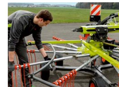
PROFIX tine arm attachment system.
