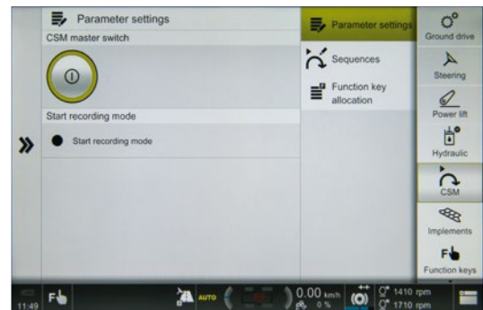
Set the parameters in the CSM overview. You can assign the function keys on the control lever as required.
