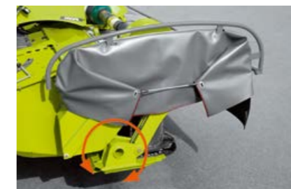
Thanks to the low pivot point, the DISCO PROFIL follows the ground contours, and not the tractor
