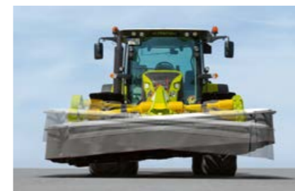
Freely pivoting suspension for accurate ground-contour following across the direction of travel
