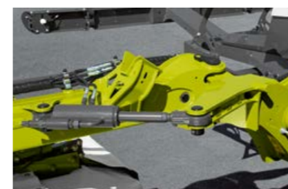
Hydraulic non-stop collision protection – in the event of a collision, the mower pivots up and over the obstacle, and resets itself automatically
