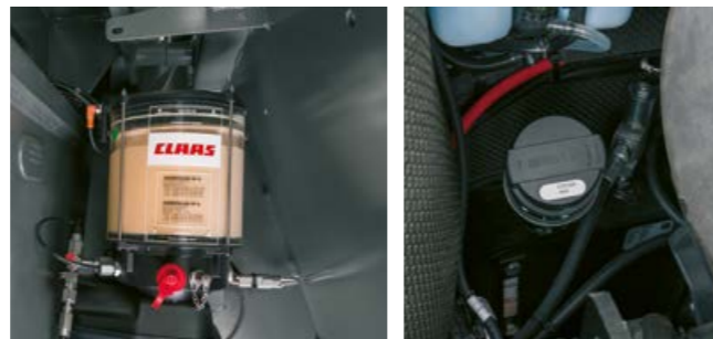
The oil filler neck for the hydraulic oil is located in a clean area under the bonnet. The oil level can be easily read directly through a clearly visible sight glass.
