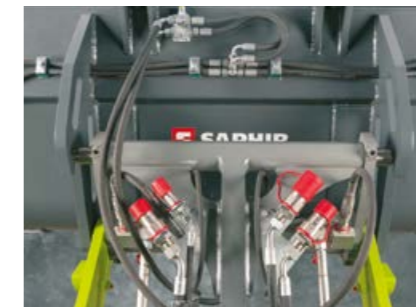
Pressure-free return at the front and an additional leakage oil pipe with connection to the implement carrier (644 / 537)
