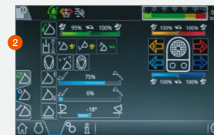
The lifting and lowering height limits are displayed on the 9" touchscreen
