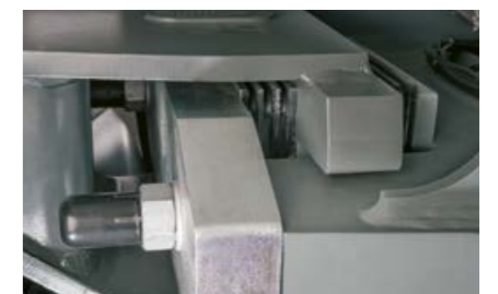
Rubber dampers in the articulated pendulum joint increase operator comfort
