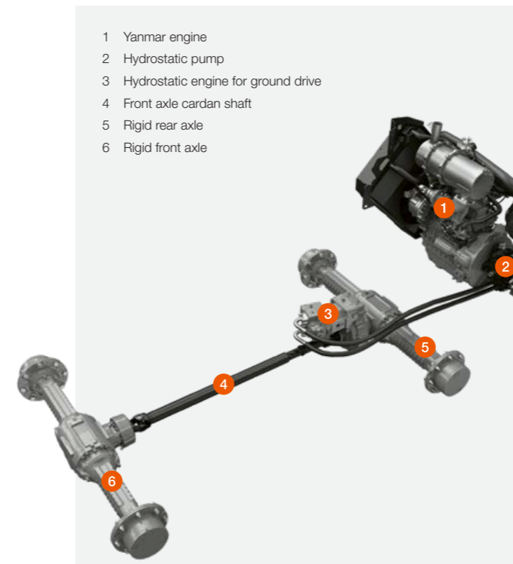
Hydrostatic transmission with self-locking braking action
