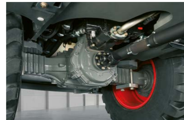
Hydrostatic transmission with self-locking braking action
