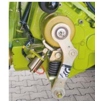
Metal detector power interrupt clutch
