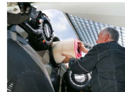
Air filter change without tools
