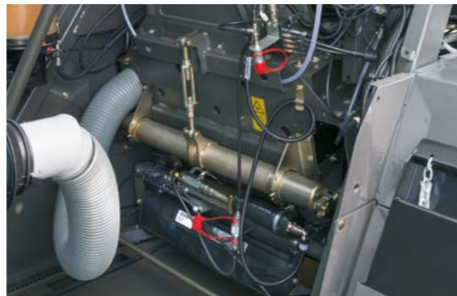
Mechanical adjustment of the crop accelerator clearance
