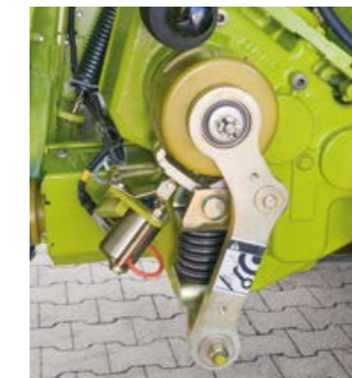
Metal detector power interrupt clutch
